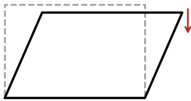
no brace: the frame can sag
